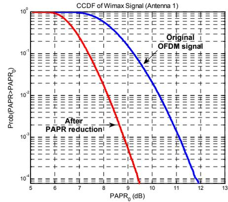
Fig. 5 CCDF showing the PAPR reduction performance of antenna 1 for a WiMAX signal
