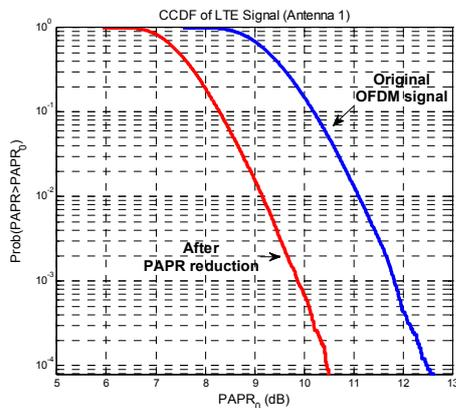
Fig. 9 CCDF showing the PAPR reduction performance of antenna 1 for a LTE signal.
