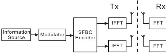
Fig. 1 Block diagram of a 2x2 MIMO-OFDM system
