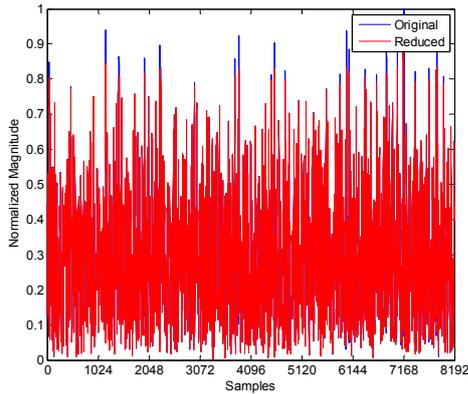
Fig. 7 Time domain signal of antenna 1 before and after PAPR reduction for a LTE signal.
