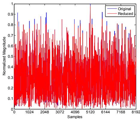
Fig. 8 Time domain signal of antenna 2 before and after PAPR reduction for a LTE signal.
