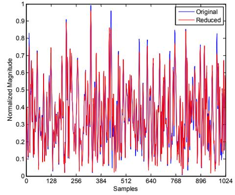
Fig. 4 Time domain signal of antenna 2 before and after PAPR reduction for a WiMAX signal.
