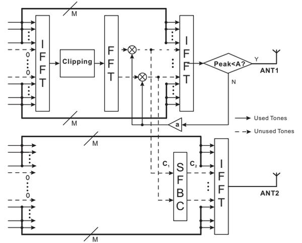
Fig. 2 Block diagram of the proposed PAPR reduction technique
