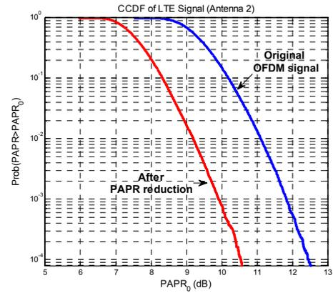
Fig. 10 CCDF showing the PAPR reduction performance of antenna 2 for a LTE signal.
