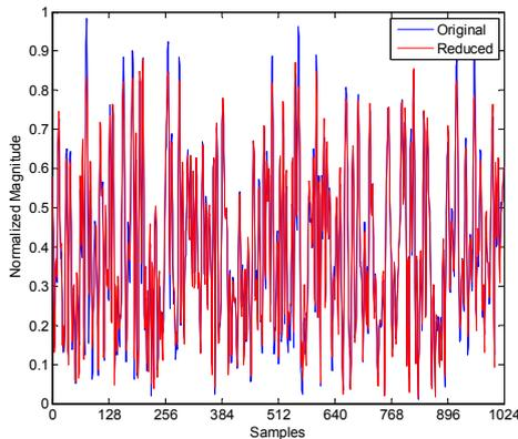
Fig. 3 Time domain signal of antenna 1 before and after PAPR reduction for a WiMAX signal.
