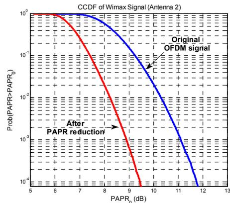
Fig. 6 CCDF showing the PAPR reduction performance of antenna 2 for a WiMAX signal
