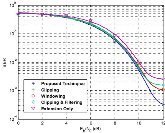
Fig. 6: BER for a WiMax system using 16 QAM. PAPR reduction is 2.5dB for all techniques shown
