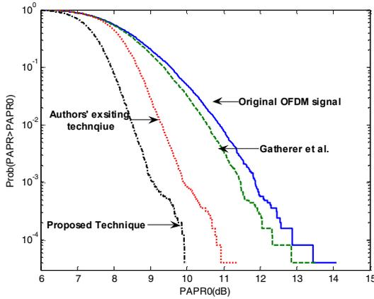
Fig. 1: CCDF plots of a 16QAM 802.11a signal.
