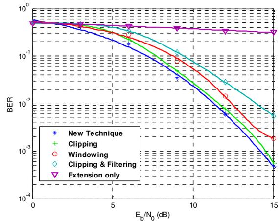
Fig. 4: BER for PAPR reduction of 5 dB for the 16QAM IEEE802.11a system
