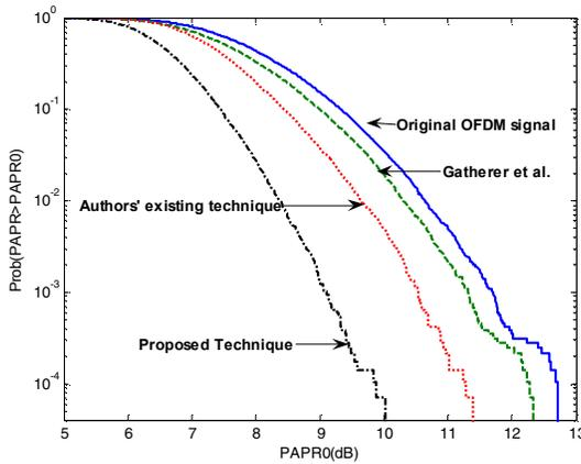
Fig. 2: CCDF plots of a 64QAM 802.11a signal.
