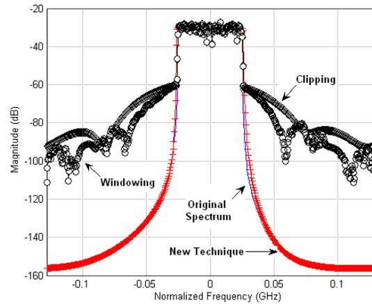
Fig. 8: Output Power Spectrum for PAPR reduction of 2.5dB for 16QAM IEEE802.16e system.
