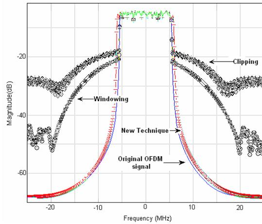
Fig. 7: Output Power Spectrum for PAPR reduction of 4dB for a 16 QAM IEEE802.11a system.
