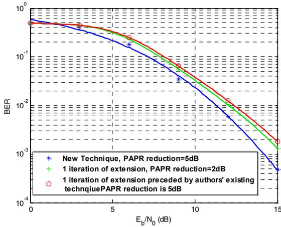
Fig. 5: BER performance comparison with different combinations of the existing technique and the extension for an IEEE802.11a system
