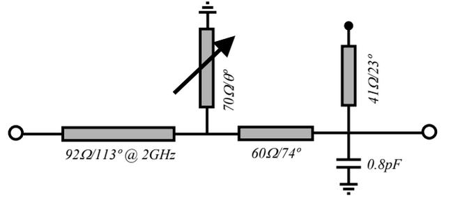
Fig. 3. Lossy distributed/ lumped test network. Stub length  $\theta$  varied over 3 values: 11°, 54°, 97°.
