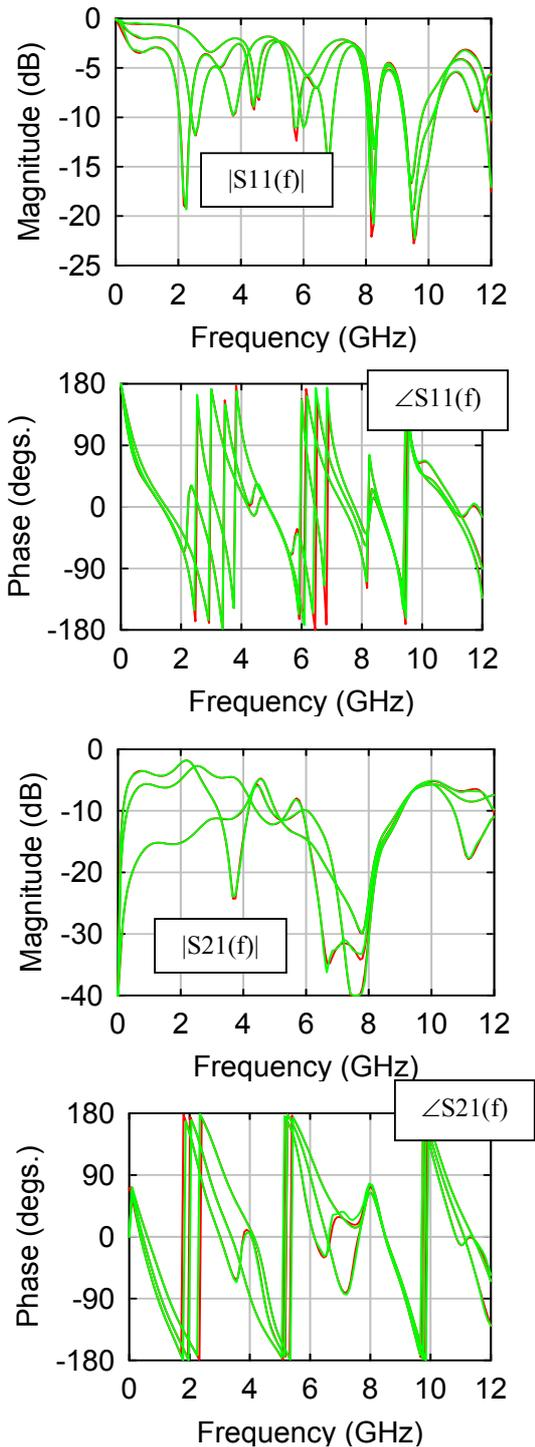
Fig. 4. Frequency domain behaviors predicted by Time-Domain description proposed in this work compared to exact response for three different stub lengths in Fig. 3 (based on 32 FD samples)
