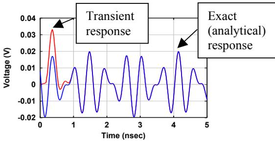
Fig. 6. Comparison between output voltage from convolution-based transient analysis (this method) and steady-state (analytical) result (2.0GHz and 2.7GHz);
