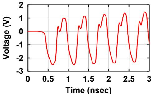
Fig. 8. Output of non-linear simulator based on method described here for amplifier in Fig. 7 at 2GHz and input drive level of 2.5V.
