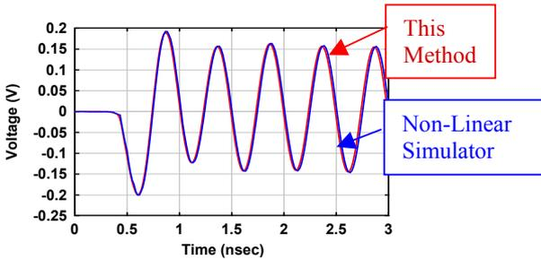
Fig. 7. Comparison between output voltage from this method and output from non-linear simulator at small input amplitude (2GHz)
