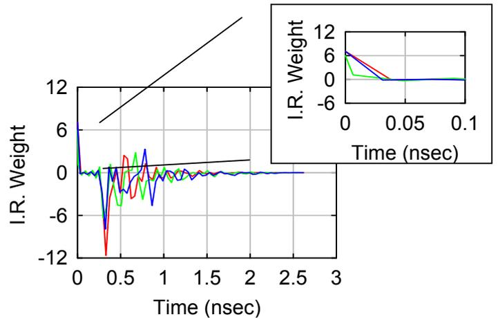
Fig. 5. Time-Domain representation of  $S_{11}(f)$  for three line lengths in Fig. 3.
