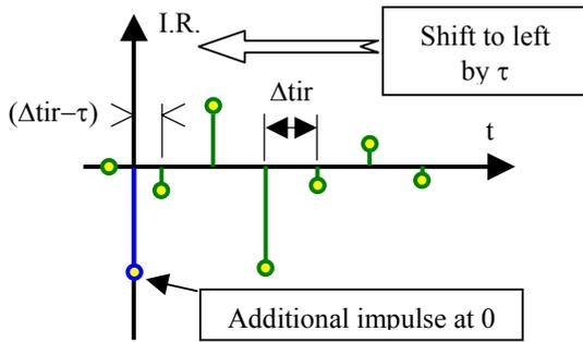
Fig. 2. Time-domain representation of Scattering Parameter  $S_{ij}(f)$  derived from response in Fig. 1.
