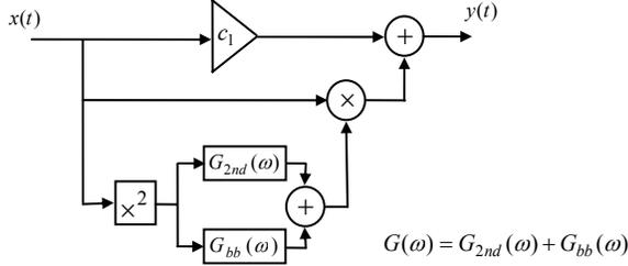
Fig. 3. Up to 3<sup>rd</sup> order model with flatness assumption at the fundamental band, and with minimal representation.
