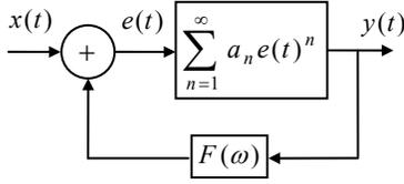
Fig. 1. Transistor model derived from physical behavior [3].
