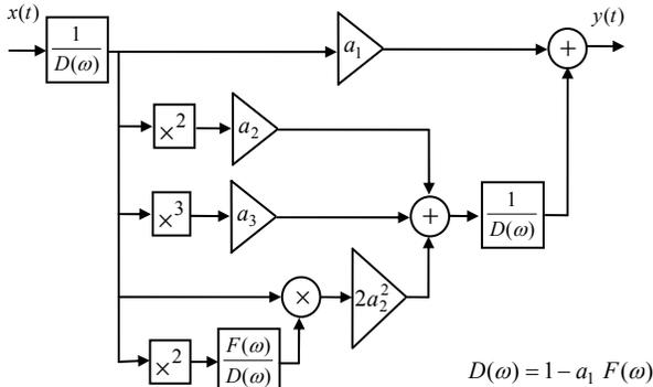
Fig. 2. Feed-forward PA model up to the 3<sup>rd</sup> order kernel.
