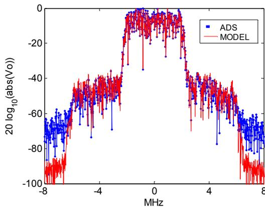
Fig. 5. Output voltage complex envelope spectrum comparison ( $P_{in}=15\text{dBm}$ ).
