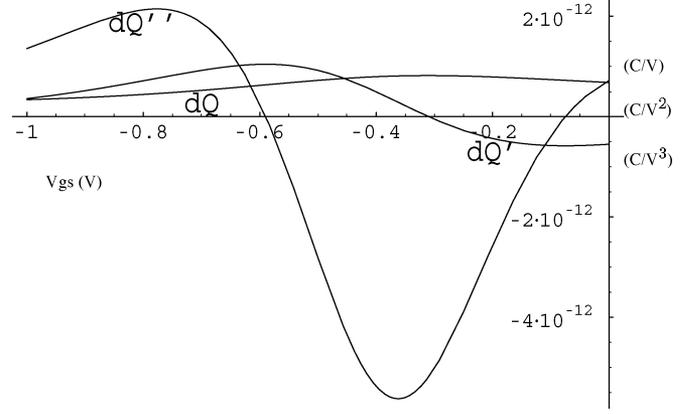
Fig. 5. Simulated derivatives of the single charge function for pHEMT model (with  $V_{ds} = 3$  V).
