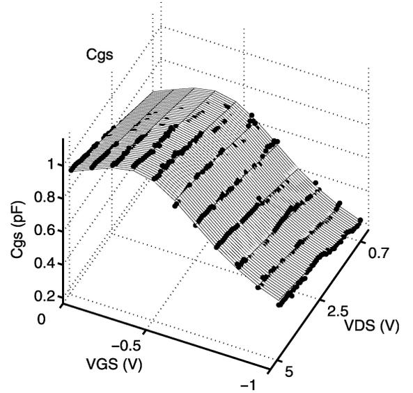
Fig. 6. Comparison of measured (dots) and modeled capacitance  $C_{gs}$  as a function of terminal bias voltages.
