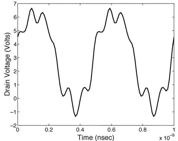
Fig. 20. Simulated intrinsic drain voltage waveform for PA when  $\eta_d = 70.5\%$ .
