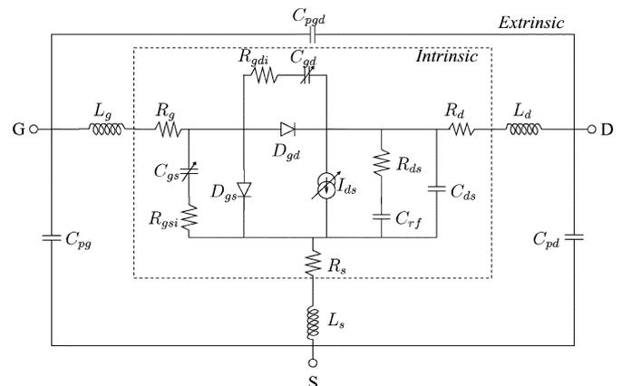
Fig. 1. Equivalent-circuit model for microwave pHEMTs.
