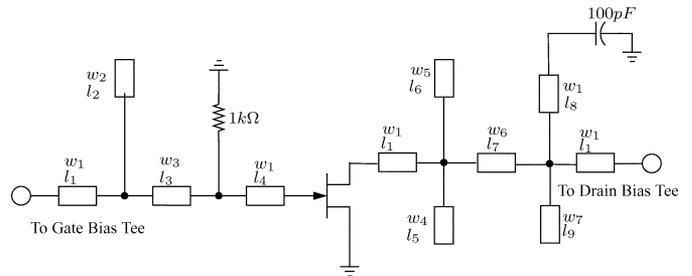
Fig. 17. Microstrip realization of PA input and output matching networks.
