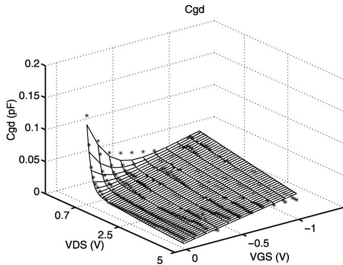
Fig. 7. Comparison of measured (dots) and modeled capacitance  $C_{gd}$  as a function of terminal bias voltages.
