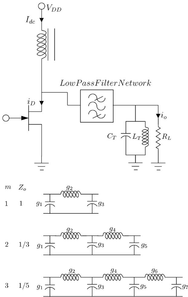
Fig. 12. Rhodes ideal low-pass matching networks for class-F PA design [4].
