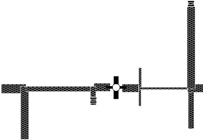
Fig. 18. Microstrip circuit layout of Fig. 17 including on-chip circuit components.
