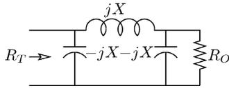
Fig. 15. Impedance inverter topology.
