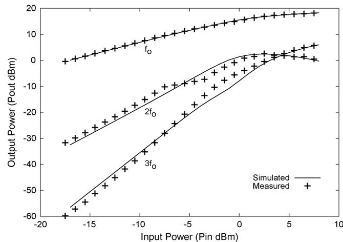
Fig. 8. Single-tone power measurements and ADS harmonic-balance simulation performance of proposed model at 2 GHz in a 50- $\Omega$  source and load impedance environment ( $V_{ds} = 3$  V,  $V_{gs} = -0.6$  up to third harmonic).
