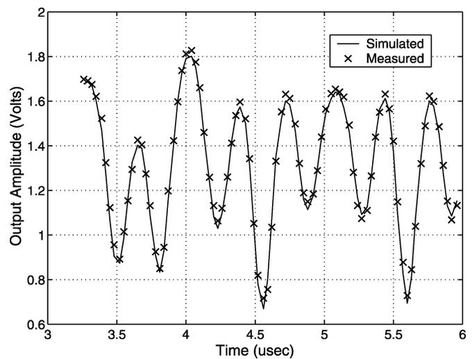
Fig. 9. Time-domain waveform amplitude of pHEMT output with W-CDMA input signal ( $V_{ds} = 3$  V,  $V_{gs} = -0.4$  V).
