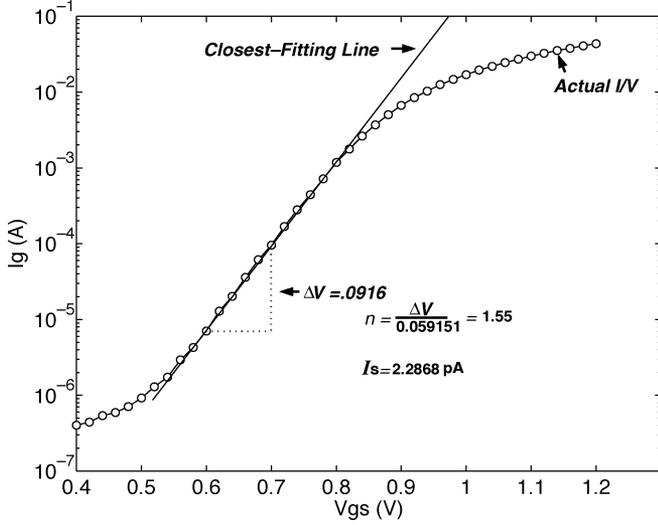
Fig. 2. Extraction of Schottky diode parameters using forward-bias gate current measurements. The ideality factor  $N$  and the gate junction current parameter were calculated to be 1.55 and 2.28 pA, respectively.
