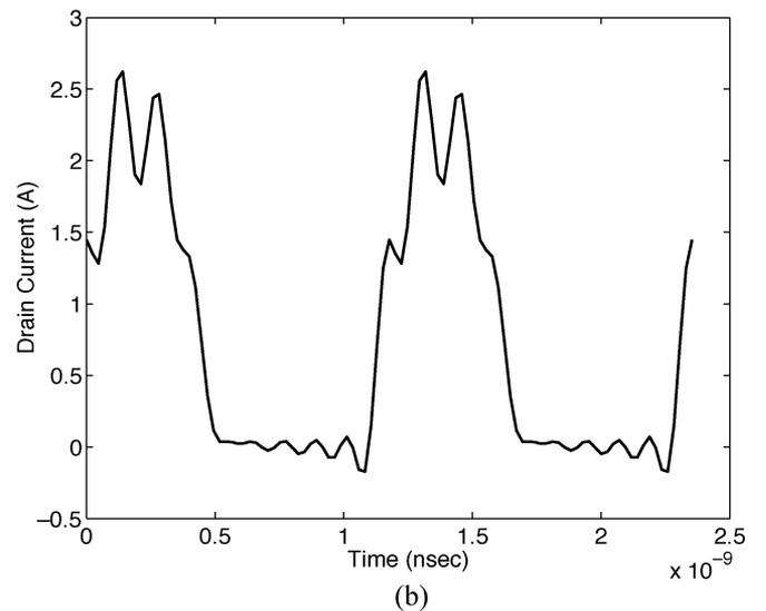
Fig. 14. Simulated class-F PA drain waveforms for ideal device case  $m = 3$ . (a) Voltage waveform. (b) Current waveform.
