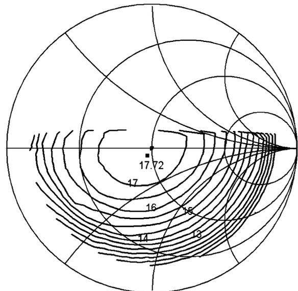
Fig. 10. Measured load-pull contours of output power (scale 0.5 dBm per contour) for pHEMT when driven at 3-dB compression point with 50- $\Omega$  source and biased at dc operating point of  $V_{ds} = 3$  V and  $V_{gs} = -0.2$  V.
