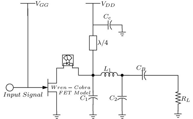
Fig. 16. Lumped class-F PA model.
