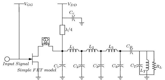
Fig. 13. Circuit topology for ideal class-F PA for  $m = 3$ .
