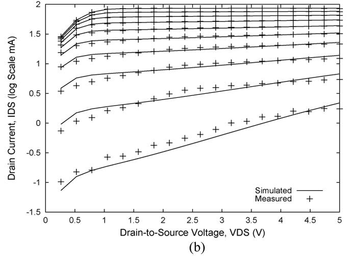
Fig. 3. Comparison between the measured and simulated dc characteristics showing: (a) an excellent global fit over entire dc bias range and (b) highlighting the COBRA model fidelity at pinchoff levels.
