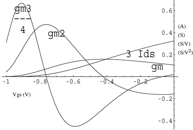
Fig. 4. Saturated drain current and its first three derivatives for the COBRA model indicating the model's excellent IMD predictive capability.
