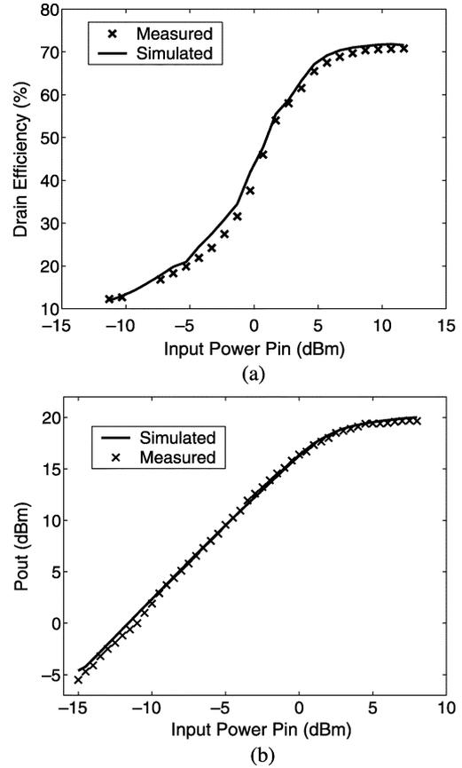
Fig. 19. Comparison between the measured and simulated: (a) drain efficiency  $\eta_d$  and (b) output power  $P_{out}$  of the class-F PA at 2 GHz with  $V_{ds} = 5$  V and  $V_{gs} = -1.0$  V.
