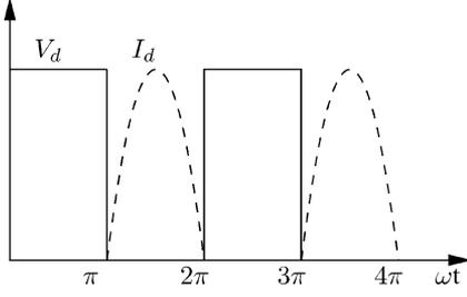
Fig. 11. Ideal drain voltage and current waveforms for the ideal class-F PA.
