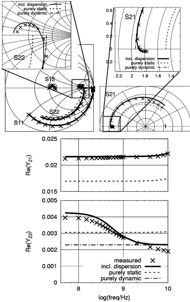
Fig. 8. Measured and modeled  $S$ -parameters (50 MHz–50 GHz) of the GaAs pHEMT under bias conditions  $Q = (0.2 \text{ V}, 3.9 \text{ V})$ . Effects of dispersion on  $S_{21}$  and  $S_{22}$  are enlarged and compared to models based on purely static and purely dynamic drain current characteristics. (Bottom) Real parts of output related  $Y$ -parameters in the lower frequency range.
