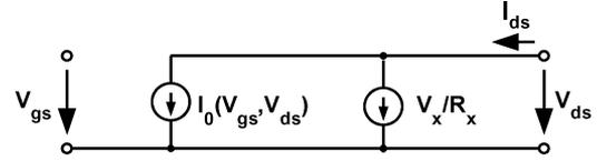
Fig. 1. Large-signal equivalent circuit of a single dispersion effect.
