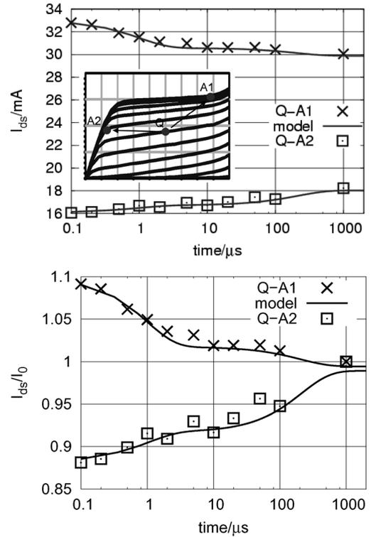
Fig. 7. Transient step response of drain current when stepping from  $Q = (0$  V,  $2$  V) to  $A1 = (0.8$  V,  $3.5$  V) and  $A2 = (0.2$  V,  $0.6$  V). Measurement (dots) and modeled values (lines).
