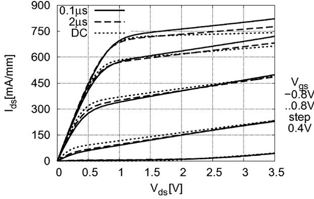
Fig. 4. Modeled dynamic  $IV$  characteristics of a  $2 \times 20 \mu\text{m}$  GaAs pHEMT based on pulsed measurements with different pulse widths.
