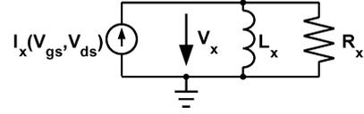
Fig. 2. Linearization of the dispersion model (dispersion source only).
