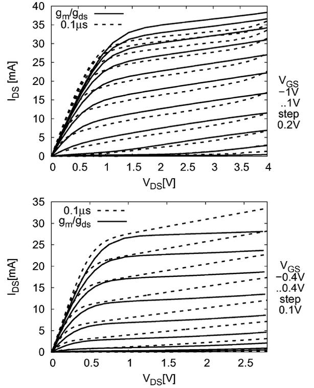
Fig. 5. Dynamic  $IV$  obtained from numerical integration of multibias transconductance and output conductance information for frequencies beyond 5 GHz. (Top) GaAs pHEMT. (Bottom) InP pHEMT. Comparison to pulsed- $IV$  with  $0.1 \mu\text{s}$  pulse width (dotted lines).
