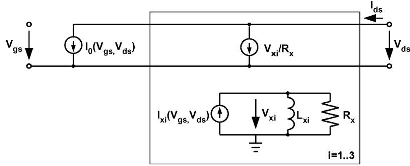
Fig. 3. Incorporation of several dispersion sources within the large-signal model topology.
