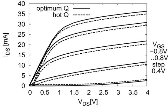
Fig. 6. “Hot” quiescent condition for numerical integration introduces essentially a shift in threshold voltage to the  $IV$  characteristics, shown here for the GaAs device.
