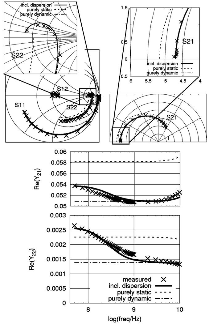
Fig. 9.  $S$ -parameters (50 MHz–50 GHz) of the InP pHEMT under bias conditions  $Q = (0.1 \text{ V}, 2.8 \text{ V})$  in a comparison to models based on dispersive as well as purely static and purely dynamic drain current characteristics. (Bottom) Real parts of output related  $Y$ -parameters in the lower frequency range.
