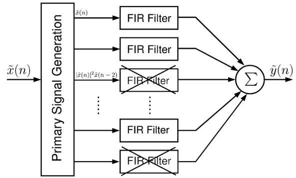
Fig. 3. Pruned Volterra series based behavioral model.
