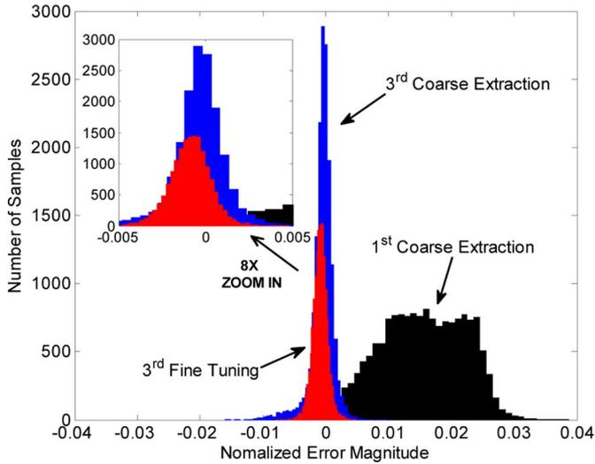
Fig. 2. Distribution of the magnitude errors between the linearized output and the original input.
