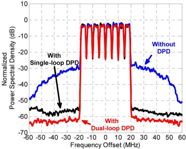
Fig. 3. Output spectra for an 8-carrier WCDMA signal with and without DPD.
