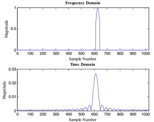
Fig. 1 Cancellation signal formed from Gaussian pulse in the time and the frequency domain
