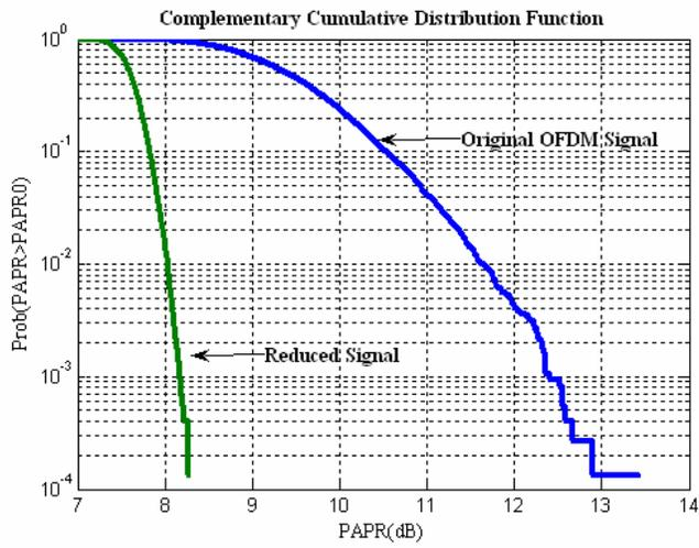
Fig. 4 CCDF plot for a WiMax signal
