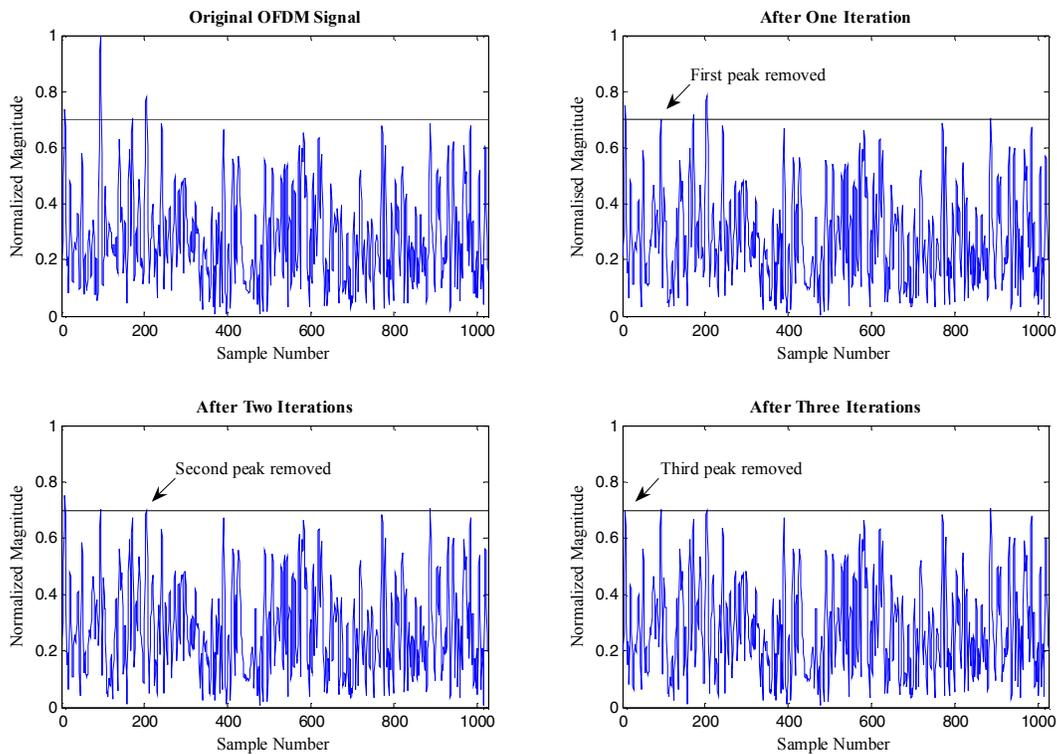
Fig. 3 Time domain sample of a WiMax signal with Tone Reservation
