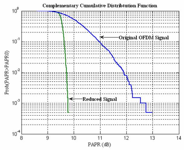
Fig. 5 CCDF plot for a DVB signal
