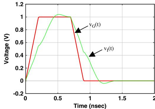
Figure 10. Pulse-transient response of the UWB antenna system in Figure 7(b) using discrete-time representation in Figure 9.
