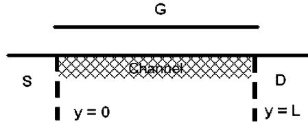
Figure 1. Simplified representation of FET physical structure.
