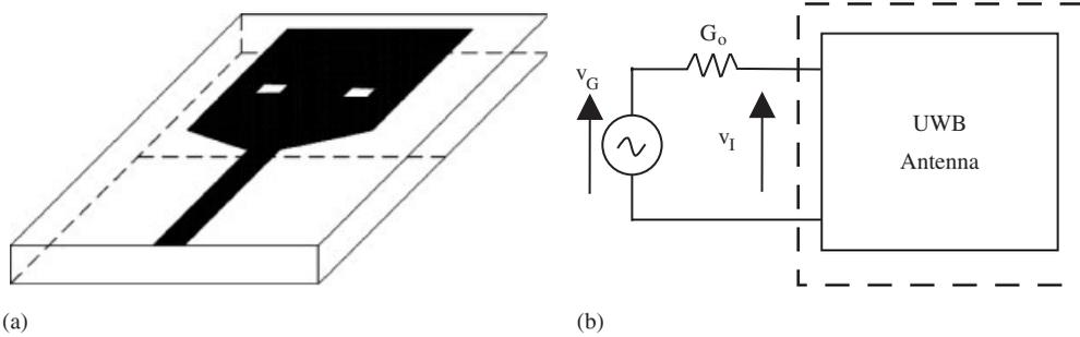
Figure 7. (a) Schematic of microstrip defected ground UWB antenna structure (substrate dielectric constant = 2.55) and (b) circuit schematic for transient analysis.
