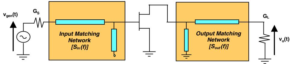
Figure 11. PHEMT amplifier incorporating non-linear device model as in Figure 5 and distributed matching/bias networks represented in discrete time.
