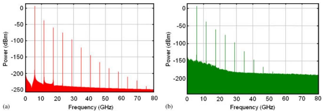
Figure 12. (a) Output voltage spectrum with single-tone input voltage at 5.8 GHz (amplitude = 2 V,  $V_{GS} = -0.2$  V,  $V_{DS} = 3.0$  V) and (b) as (a) with channel noise introduced directly as signal generator.
