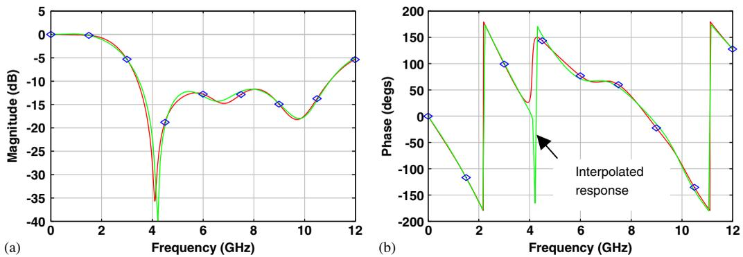
Figure 8. Reflection scattering parameter of the UWB antenna as a function of (a) frequency and (b) magnitude phases. Points indicate samples used to construct discrete-time impulse response. Interpolated and exact (EM) responses compared.
