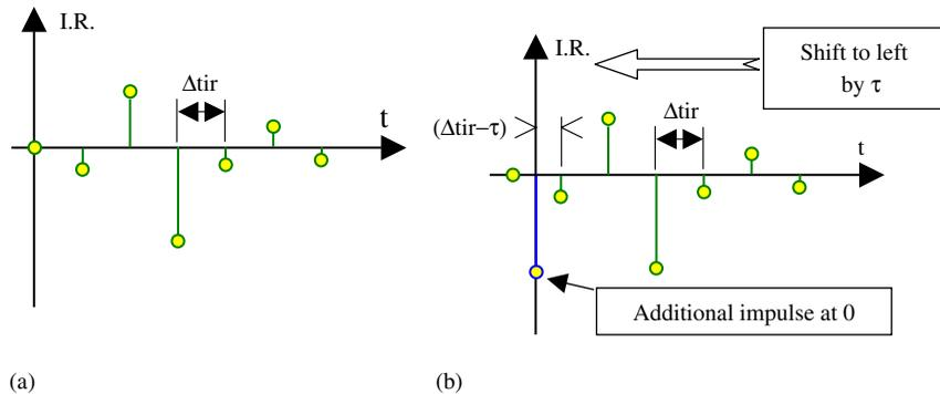
Figure 6. (a) Time-domain representation of periodic extension of  $F_{ij}(f)$  in Equation (8), satisfying both conditions (1) and (2). (b) Time-domain representation of scattering parameter  $S_{ij}(f)$  derived from response in (a).
