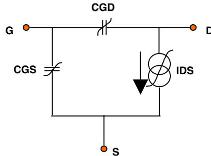
Figure 2. Core elements of intrinsic FET equivalent circuit model.
