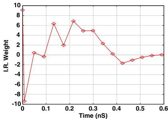
Figure 9. Discrete-time representation of reflection scattering parameter of the UWB antenna using frequency samples shown as points in Figure 8.
