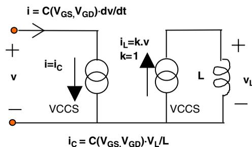
Figure 3. Using circuit elements to allow non-charge-based implementation of non-linear capacitance.
