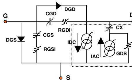
Figure 5. Advanced FET equivalent circuit model including additional elements to model dispersion in drain current.
