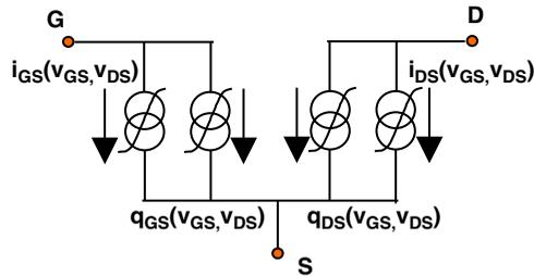
Figure 4. Basic topology of table-based FET non-linear model.
