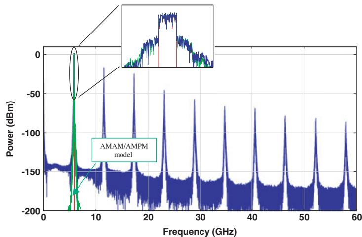
Figure 13. Broadband output voltage spectrum with 64-channel OFDM signal, each channel modulated with 64-level QAM. AMAM/AMPM behavioural model shown for comparison (in the first zone).
