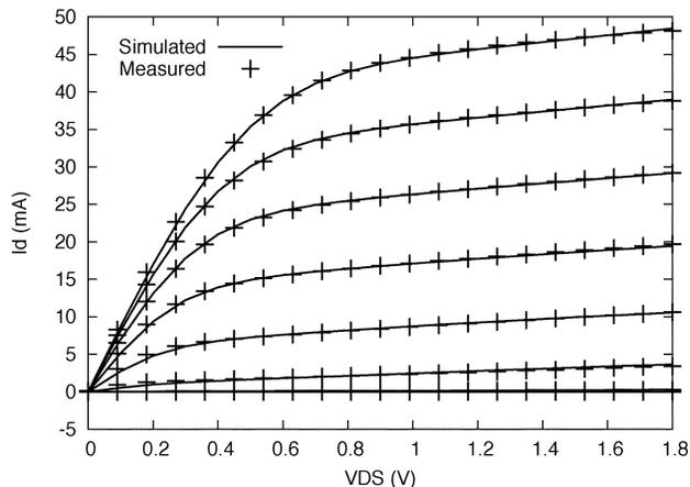
Fig. 1. DC characteristics for  $V_{GS} = 0$  to 1.6 V in steps of 0.2 V.
