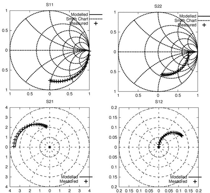
Fig. 2.  $S$ -parameter measurements and simulations for  $V_{DS} = 1.0$  V and  $V_{GS} = 0.8$  V from 0.5 to 10 GHz.
