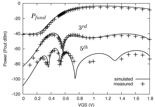
Fig. 4. Characteristics of intermodulation distortion products against swept gate-source voltage for weak-signal two-tone tests at  $V_{DS} = 1.0$  V and  $P_{in} = -15$  dBm.
