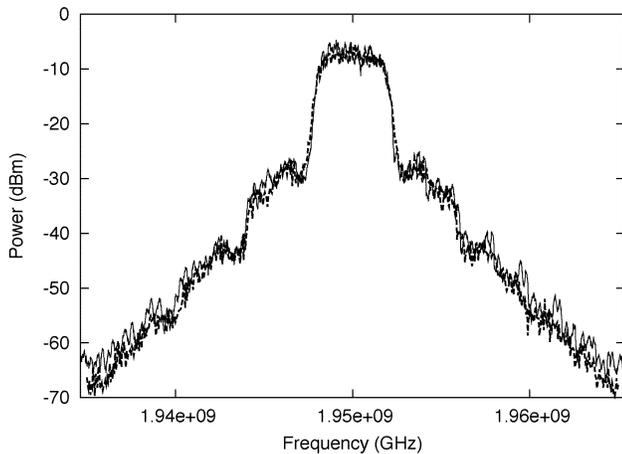
Fig. 6. Measured and simulated frequency spectra of a WCDMA signal of  $P_{in} = +4$  dBm at  $V_{DS} = 1.0$  V,  $V_{GS} = 0.8$  V.
