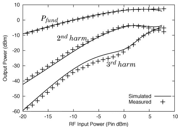
Fig. 3. One-tone power measurements against ADS simulations for the extracted model at  $V_{DS} = 0.8$  V and  $V_{GS} = 1.2$  V.
