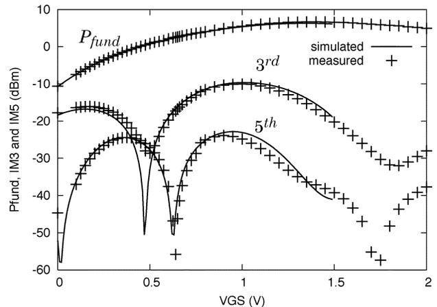
Fig. 5. Characteristics of intermodulation distortion products against swept gate-source voltage for two-tone tests at  $V_{DS} = 1.2$  V and  $P_{in} = -2$  dBm.
