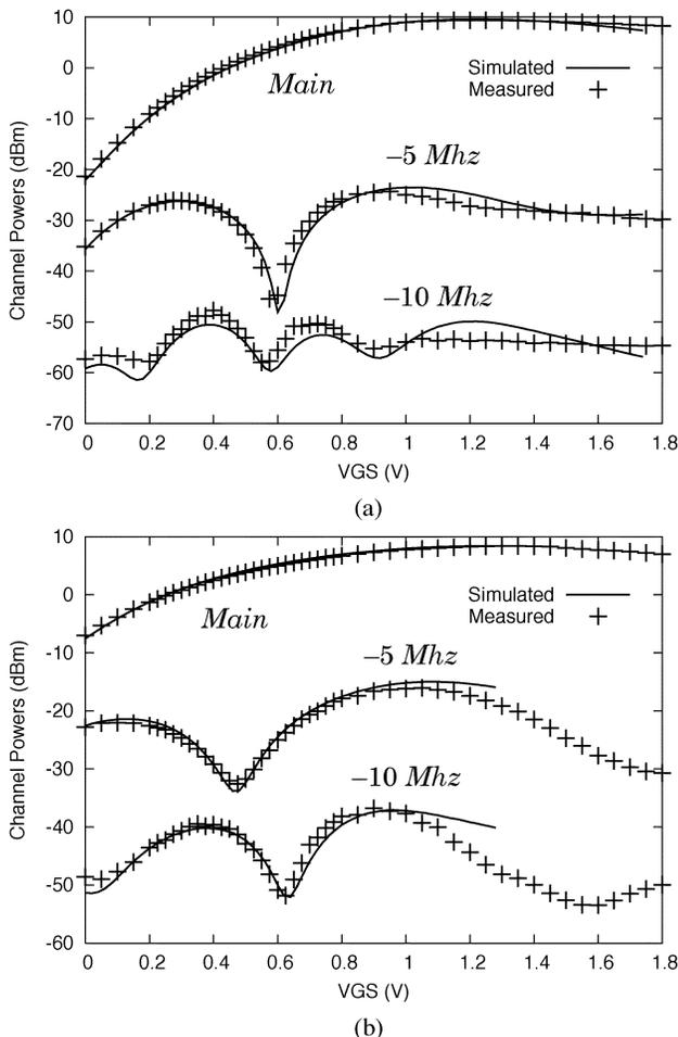
Fig. 7. Simulations versus measurements of the main and lower channel powers for swept  $V_{GS}$ , for a WCDMA signal of high input power applied to the MOSFET at (a)  $V_{DS} = 1.6$  V,  $P_{in} = -2$  dBm, and (b)  $V_{DS} = 1.0$  V,  $P_{pin} = +2$  dBm.
