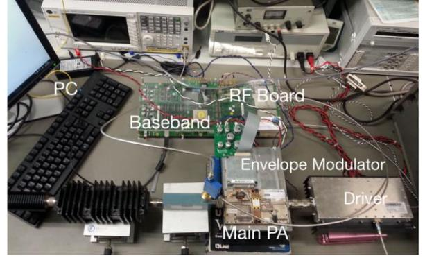
Fig. 4. The envelope tracking PA test bench.
