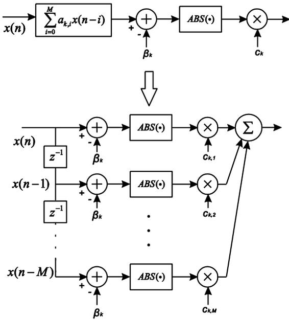
Fig. 2. Modification of the basis function.
